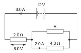
What is the current in resistor R and what is the p.d. across resistor R?
